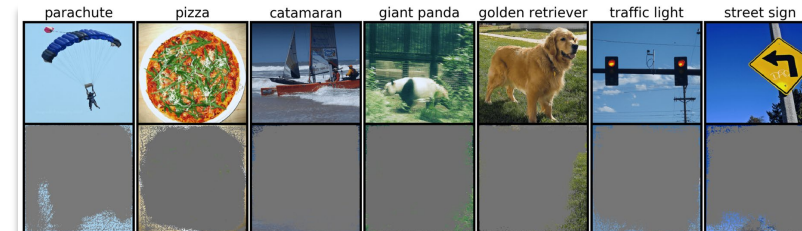
Figure 4: Sufficient input subsets (threshold 0.9) for example ImageNet validation images. The bottom row shows the corresponding images with all pixels outside of each SIS subset masked but are still classified by the Inception v3 model with \geq 90\% confidence.
